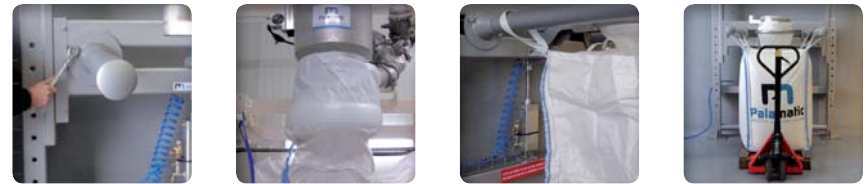
Hooking forks width adjustment allows conditioning of all types of big bags Inflating seal to insure dust containment for a clean work area Tension cylinder insures a perfect big bag filling and handling stability Big bag removal with fork or pallet truck
