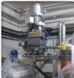
Cyclone transfer system with dosing device
