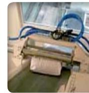
**Pre-crushing of the bags** when passing bags with lumps. The passage of the bag in front of the detect sensor starts the crushing action
