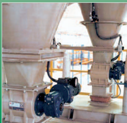
Valves under silos
